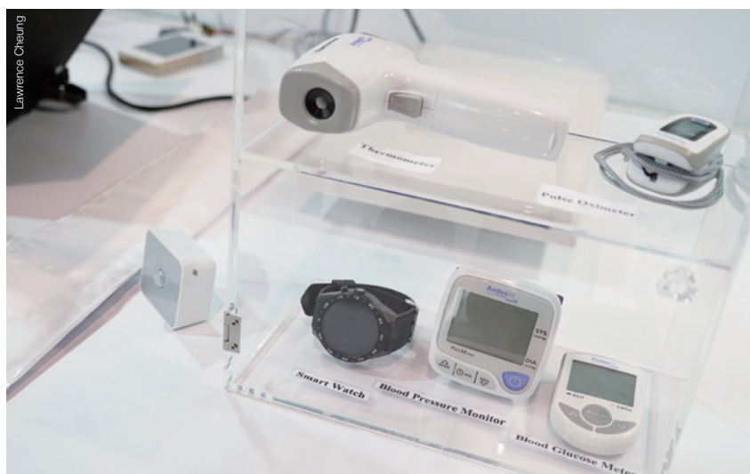
樂齡護理監察系統收集院友的實時健康資訊，利用智能傳感器追蹤院友的實時位置，確保院友安全。The Gerontech Health Care Monitoring System collects real-time health data of elderly home residents. Smart sensors are also used to track and trace the real-time location of residents to ensure their safety.
