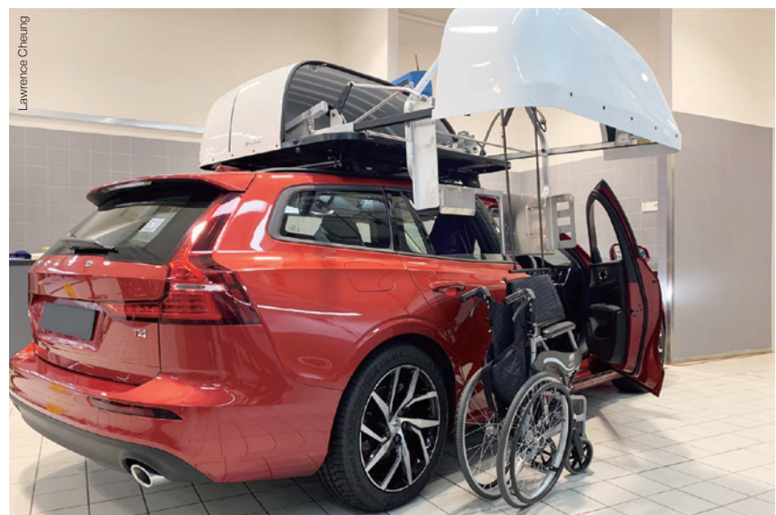
生產力局轄下的汽車科技研發中心提供技術支援，讓輪椅使用者在駕駛時亦可將輪椅自助存放於車頂。 Hosted by the HKPC, the Automotive Platforms and Application Systems R&D Centre offers technical assistance such that wheelchair users could help themselves to store their wheelchairs on top of their cars.
