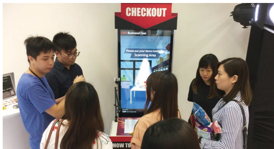
只要將商品逐一放在收銀台，兩旁的鏡頭就會透過影像分析自動輸入到付費清單。 The customer simply places the items one by one at the checkout counter and the cameras on both sides automatically input those items into the payment list through image analysis.
