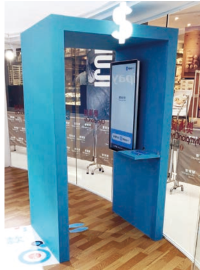
顧客把貨品置於感應器，就可一次過結算。顧客如若把未付款貨品帶離無人店，出口會響起警報。 Customers can check out at once by placing chosen items on the sensor. The entrance alarm will be triggered if customers leave the unmanned store with unpaid items.
